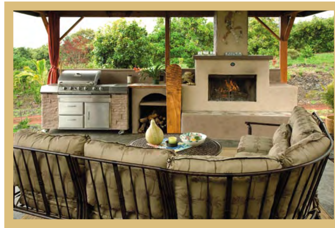
To create the outdoor fireplace, a wood frame was built around a pre-fabricated fireplace, which was then stuccoed. John created the tiled chimney gecko and hearth. Lanai furniture from Champagne Spa & Lanai.
